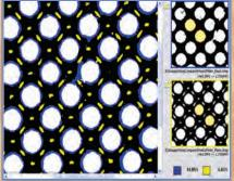
COLOR SEPARATION ANALYSIS from printed halftones, separated and analyzed for true halftone dot area analysis & correction. Useful for gray balance control and for printing without targets.
